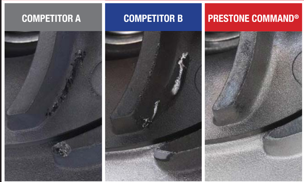
DIRECT COMPARISON WATER PUMP TEST - MODIFIED ASTM D2809 100 HOUR TEST
